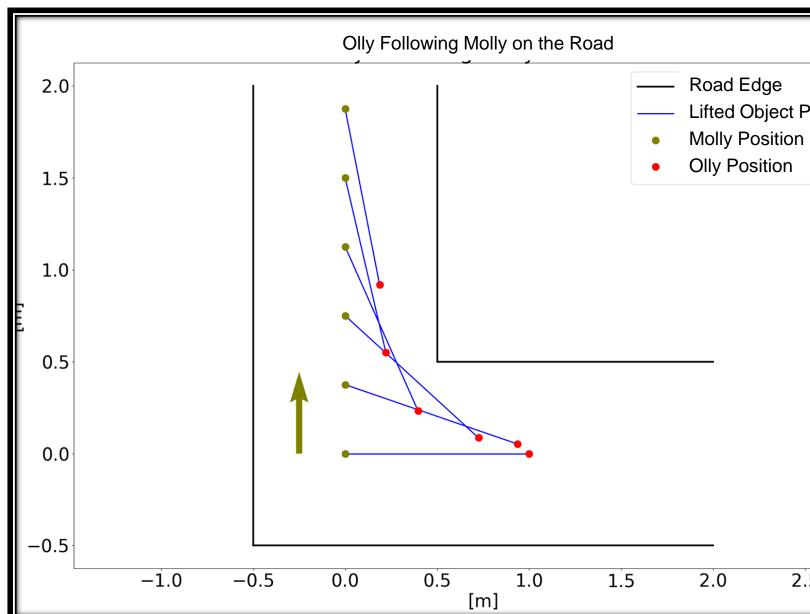
Using the SLAM map, a model predictive control ("MPC") optimization problem determines Olly's behavior. By predicting Molly's future behavior, Olly's controller computes a trajectory that maintains a specific distance from Molly and avoids obstacles. The picture above shows Olly's path given a simple trajectory for Molly.
