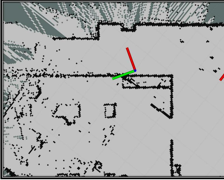
We use a Simultaneous Localization and Mapping (SLAM) algorithm to turn the LIDAR point cloud into a map of the robot's surroundings. The image shown above is a map that we built of the basement of Hesse Hall. The darker a line is, the more confident the robot is that that region is a solid wall.
